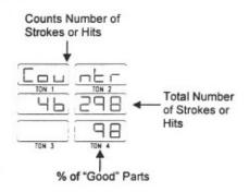
The Counter Reset Display is shown below: NOTE: Press the RIGHT ARROW key & ENTER key to reset to zero.
