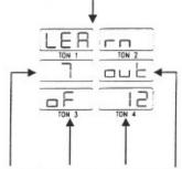
The unit keeps track of how many parts have been made. In this example, the display reads "7 out oF 12" across four windows, meaning "7 parts out of 12 parts have been made."
