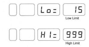
If the resolver shaft RPM is between the motion limits inclusively, the motion output will be enegized. Motion limits are common for all 16 programs.
