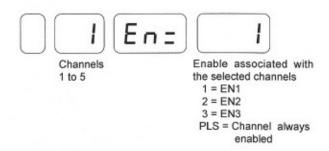
Enables EN1, EN2 and EN3 are user assignable to channels 1 to 5. These enable inputs are read during the period between the new cycle position and the next setpoint position for that channel. If a true level is read then the channel associated with that input is enabled for that cycle.
