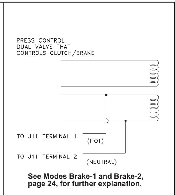
**Figure 12 - Brake Wiring**
