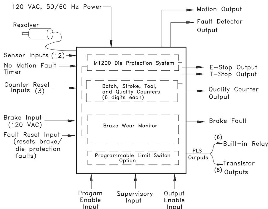
**Figure 1 - M1200 Block Diagram**
