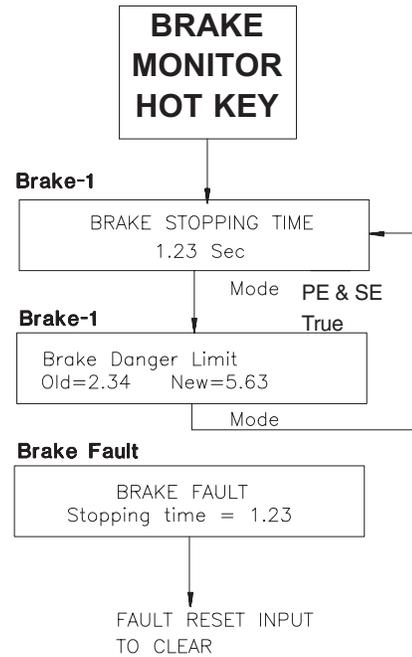
Figure 17 - Brake Monitor Hot Key Menu
