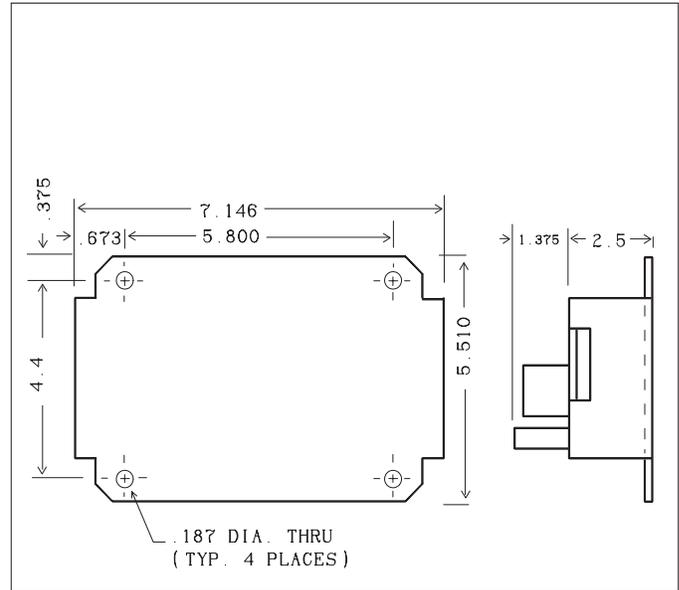
**Figure 5 - Power Relay Output Chassis, 8-Channel**
