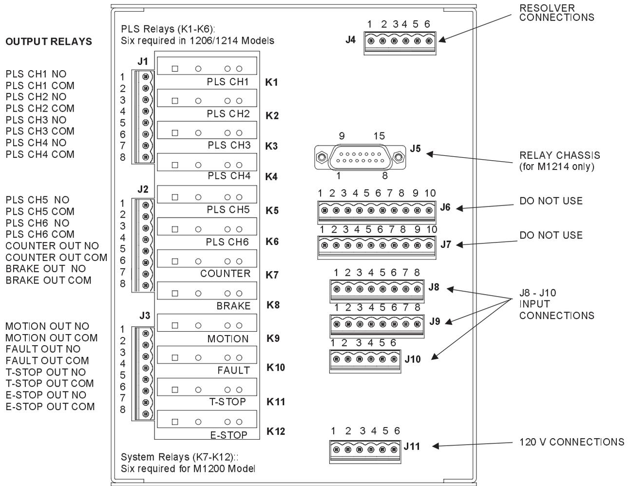
**Figure 7 - M1200 Back Panel Wiring**
