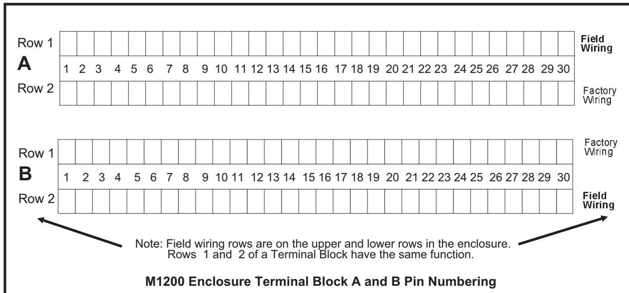
**M1200 Enclosure Terminal Block A and B Pin Numbering**
