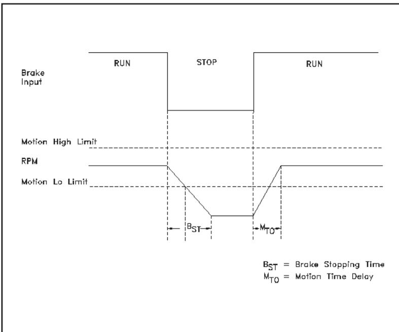
**Figure 11 - Brake Stopping Time and No Motion Detect Timer**
