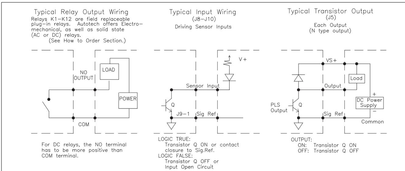
**Figure 8 - Input and Output Types**
