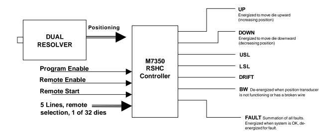
When the M7350 RSHC Module is used with the A120, Quantum, MF1, and MF2 cradles, it is not possible to access remotely each of the 500 dies, but that function is always available by programming through the use of registers.
